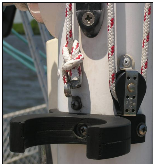
The pole chock and fittings for the up/down line.
