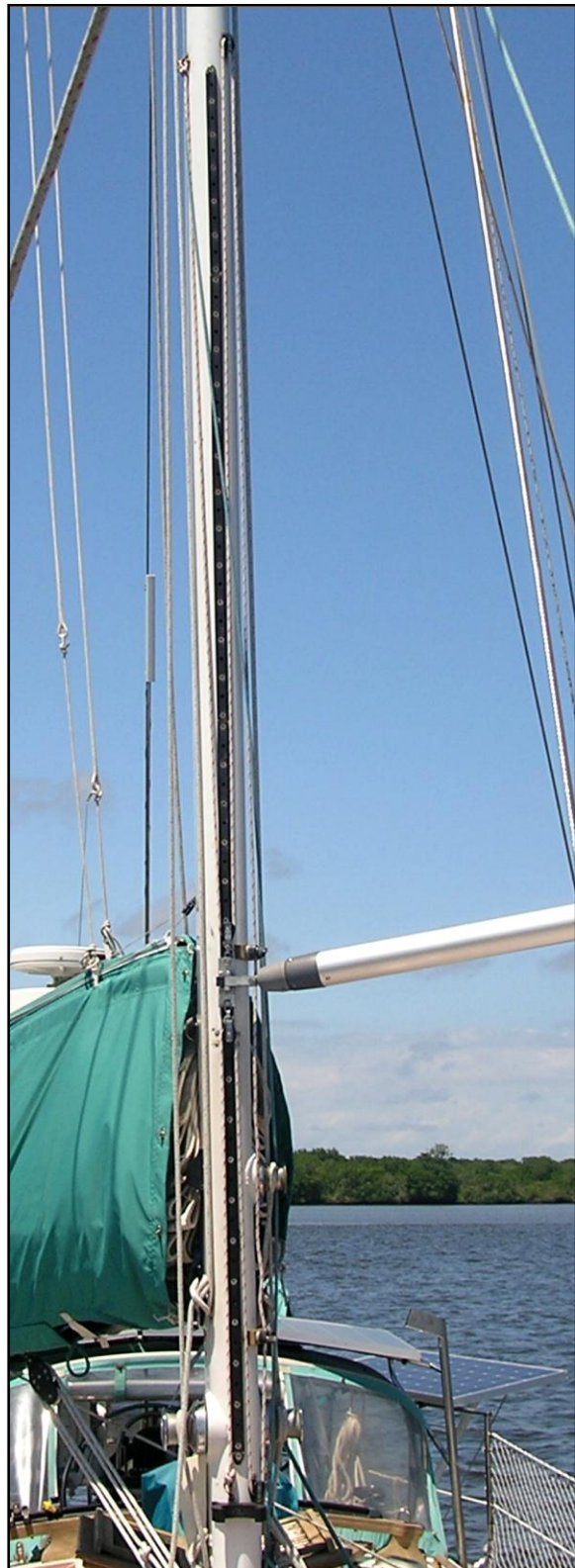
The pole and track in use. The inboard end of the pole can travel up and down on the track, controlled by a single line cleated on the mast.
