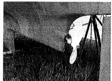
Below, on the left is a picture of the keel profile, which shows it's low aspect nature and shallow draft. The picture on the right shows the full bilges and flat underbody of the center sections of the hull. This keel and hull configuration allows The vessel to cruise in shallow water while still providing a stiff hull that can stand up to a relatively large sail plan.
