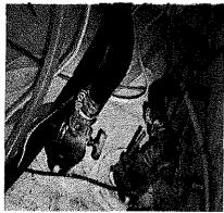
The through hulls in the head compartment (above, left) consist of one 1-1/4" seacock that provides the overboard discharge for the holding tank and a 3/4" seacock that provides the drain for the sink and seawater input for the toilet and the deck wash-down pump.
