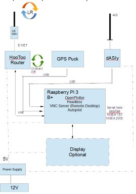
The dAISy 2+ device provides AIS info as well as NMEA 183 I/O, currently the AIS antenna is not mounted but will be soon. The AIS data is displayed on the Chart plotter and can be enabled to define collision warnings as needed.
