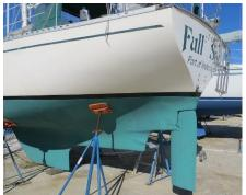
This picture shows the skeg and rudder configuration as well as a close up of the gudgeon that holds the rudder to the skeg. This configuration provides a partially balance helm and relatively effortless steering, eliminating any need for wheel steering on. The gudgeon is made up of two bronze pieces that wrap around the rudder shaft where it is exposed in the notch in the rudder. The gudgeon is through-bolted to the rudder skeg. As
