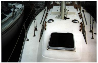
To open the hatch, rotate the handles outward until they are parallel to side edges of the hatch. This releases the cams that secure the hatch cover. Pushing or pulling the cover upward to one of the rollstop positions opens the hatch. The Hatch may be secured in two positions: fully sealed and ventilation. To fully seal the cover pull or push it fully down so that the gasket in the cover is pressed against the frame then turn the handles inward until they are
