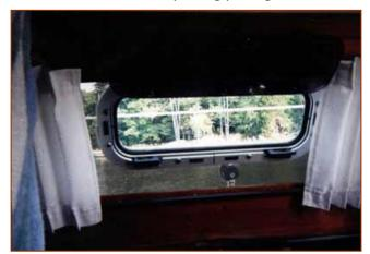
compartment for a total of six ports, three on each side of the trunk cabin. The aft portlights on each side are 4"x14" and the remaining four portlights are 4"x10". Two cam dogs on the lower edge of the lexan window secure each portlights. The handles on the dogs are turned inward so that the cams slide into the slots on the portlight frame the window is pushed against the gasket on the frame providing a watertight seal.
