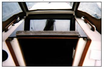
The companionway hatch consists of a sliding hatch cover and removable drop slides (see figure 1). This hatch provides the main access to the cabin from the cockpit. The hatch is protected by the canvas dodger and thus can be left open most of the time while underway, at anchor, or tied to the dock. This is the largest opening into the cabin and provides the primary ventilation.
