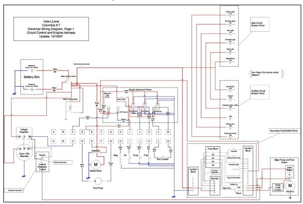
All of the circuits are controlled and distributed from one of three circuit breaker/switch panels. Full Sail was delivered with a single breaker panel with a battery selector switch, which is located above the galley sink, and depicted at right. On the right side of the panel are the battery selector switch and the battery voltmeter. This switch controls only the output of the batteries, not the charging circuits. The Newmar battery charger is wired
