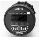
Just outboard of the auxiliary panel is a Link 10, which measures the current delivered by the batteries to the active circuits on the boat. I use this ammeter to monitor the current usage while at anchor or under sail. It is also a useful tool in diagnosing refrigeration problems.
