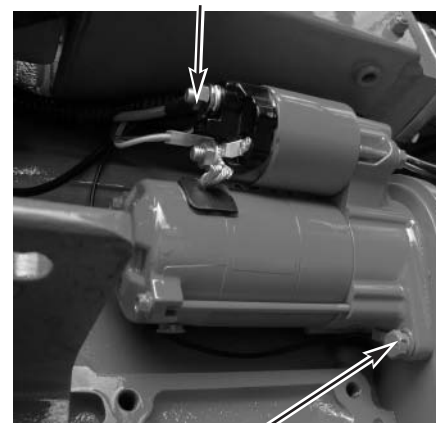
Typical start battery negative
