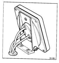
**Note:** Because the instrument breathes through the vent in the rear case, this bracket is for interior use only.
